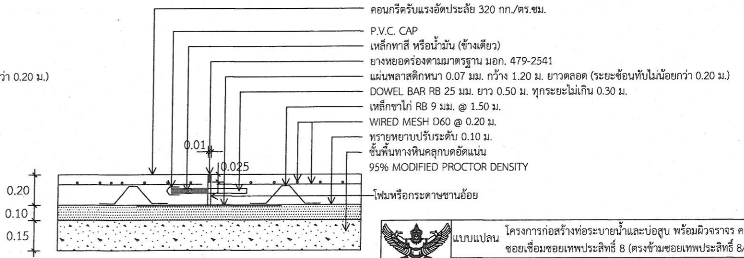
DETAIL OF EXPANSION JOINT
